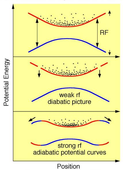
Atoms with energy >h( $v_{rf}$ - $v_0$ )/2 evaporate!
