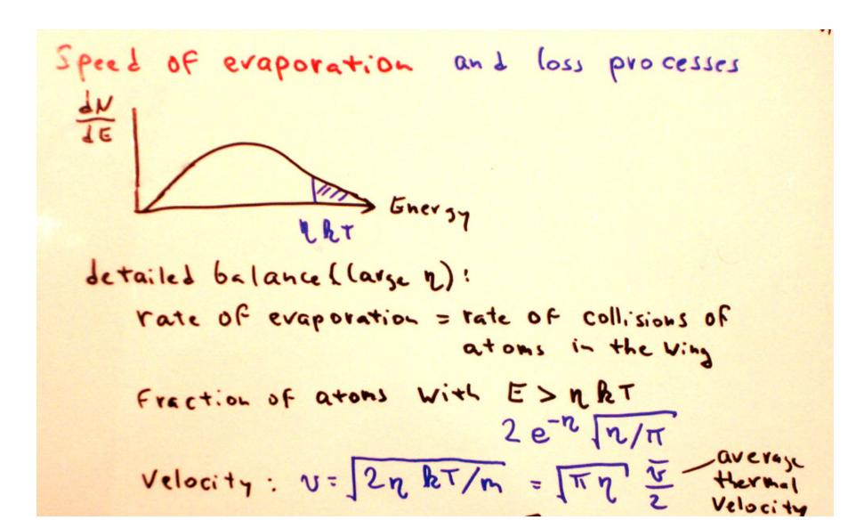
Speed of evaporation and loss processes detailed balance (large n): rate of evaporation = rate of collisions of atoms in the Ving Fraction of atoms With E>n RT 2e-n/17/11 Velocity: U= 2n RT/m = TTT & Hermal Velocity N = - no 5 v [N.2. e-2 /2/1 = - N/Tev Compare to = no 5 V TZ
