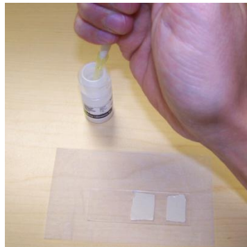
Figure 6.1 Beads are diluted using a pipette and placed between strips of double sided tape
